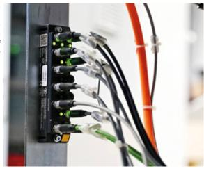
Turck's I/O components with decentralized control logic move the required intelligence to the direct environment of the conveying line
