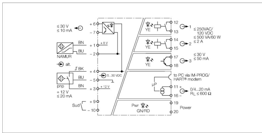
The rotation speed monitor IM21-14-CDTRI analyses frequencies, rotation speeds and pulse trains of rotating motor, gear or turbine parts according to over or undershoot of adjusted limit values. The current value is indicated on a display on the front of the device.
