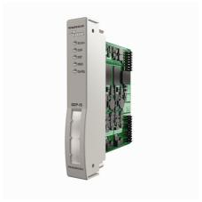
The GDP-IS gateway serves to connect the excom® system to PROFIBUS-DP networks. Connection to the PROFIBUS-DP is established via optical fibers or copper cables. When using optical fibers for data transfer an optocoupler pair must be installed between wired and optical PROFIBUS which also adapts the level to the IS layer. When using copper cables a segment coupler (RS485-IS coupler) must be installed to ensure explosion protection.
