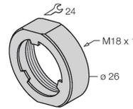
Protective nut for M18 × 1 threaded barrels; material: Stainless steel A2 1.4305 (AISI 303)
