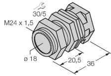
Quick-mount bracket with dead-stop; material: Chrome-plated brass. Male thread M24 × 1.5. Note: The switching distance of the proximity switches may change when using quick-mount brackets.
