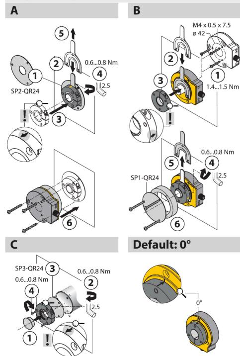
The extensive range of mounting accessories enables easy adaptation to many different shaft diameters. Due to the measuring principle, which is based on the functional principle of an RLC coupling, the encoder is immune to magnetized ferrous chips and other interferences. As a result, there are few possible causes of error during mounting. The adjacent figures show the simple installation of the two separate units: the sensor element and the positioning element: Mounting option A:
