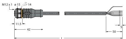
Dimension drawing Type ID RKC5701-5M 6931034
