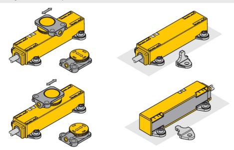
Extensive mounting accessories provide various proportions for installation.
