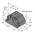
Floating positioning element for linear position sensors LI-Q25L; the nominal distance to the sensor is 1.5 mm; pairing with the linear position sensor at a distance of up to 5 mm or misalignment tolerance of up to 4 mm.
