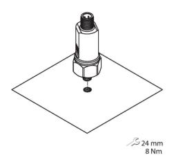
Using an M8 screw-in thread, the vibration sensors can be easily screwed into the component to be monitored and fastened into place.
