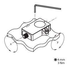
The measuring principle used makes mounting and commissioning the device easy, e.g. because being adjacent to metal does not interfere with the measuring principle.
