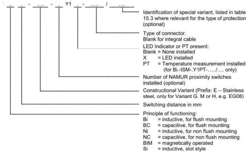
The range of two-wire proximity switches type ...-...-Y1-.../... consists of different designs divided into ten groups. The identification of the appropriate type group is related to the designs and can be determined from the following table:
