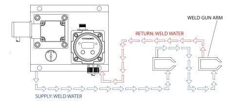
3.3.1.3 Weld Gun with Transformer Parallel Installation
