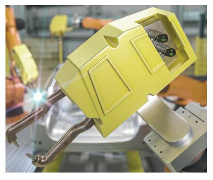
Monitoring the cooling circuit on welding clamps
