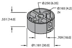
Positioning element P2-RI-QR20, operating at a distance of 0-5 mm to the sensor surface. Nominal distance is 1 mm.
