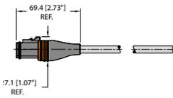
Overmolded Deutsch connector cable for the US, DT06-3S-1876-\*M
