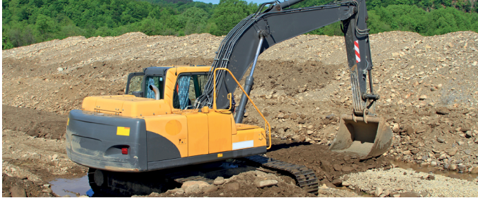
Inclination measurement on the bucket, boom, and undercarriage for optimal control
